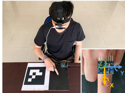
Figure 6: The experimental setting in experiment two. A participant touched on the touch screen with an IMU ring. The subfigure shows the coordinate of the IMU ring.
